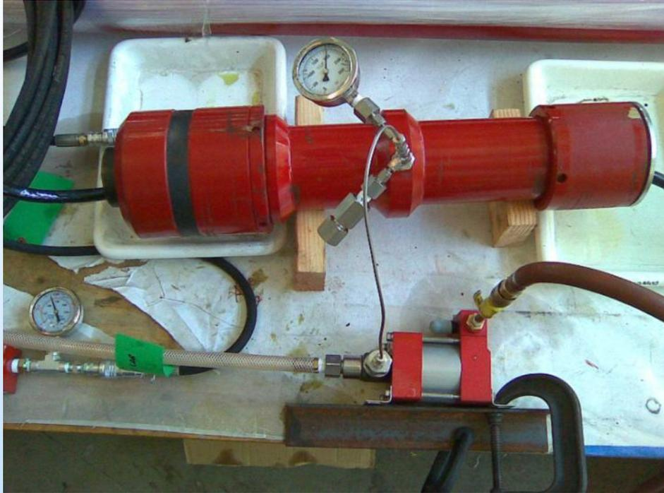
Pressure testing of polyurethane
